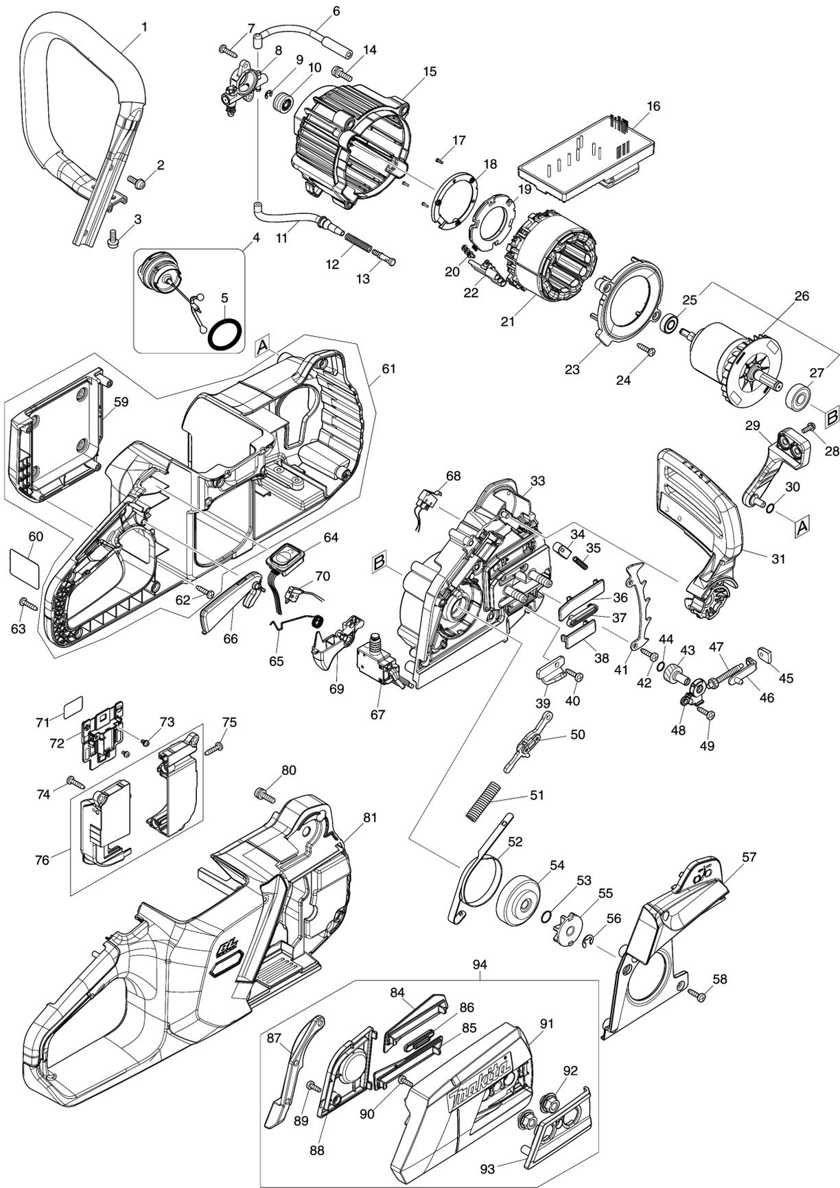
Model No.UC011G 350MM CORDLESS CHAIN SAW
